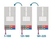
Each A2C-D75 decoder output module enables 75 stations, and allows up to three two-wire paths to the field. You can easily connect more than 75 stations to a single wire path, by assigning stations from one module to another.
