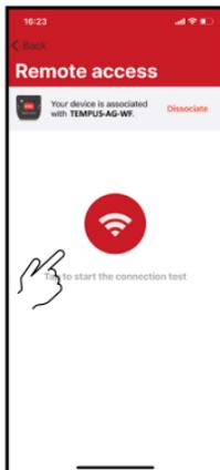
3. Push the red button to test the connection LoRa™
