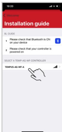
Select the required TEMPUS-AG-WF to be installed from the list of the available devices
