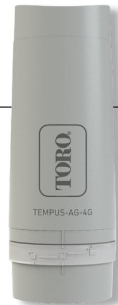
**4G - LoRa™ Gateway to connect and control up to 25 field modules via LoRa™.**
