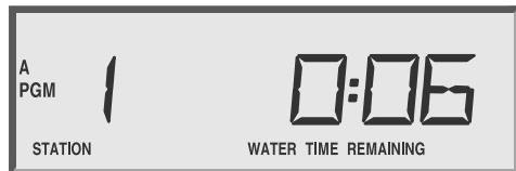
2. Press PGM until the program using the desired station is displayed.
