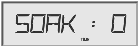
6. Use the arrow keys to set the minimum soak time from 1 to 99 minutes.
