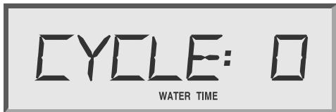
4. Use the arrow keys to set the maximum watering time from 1 to 99 minutes.
