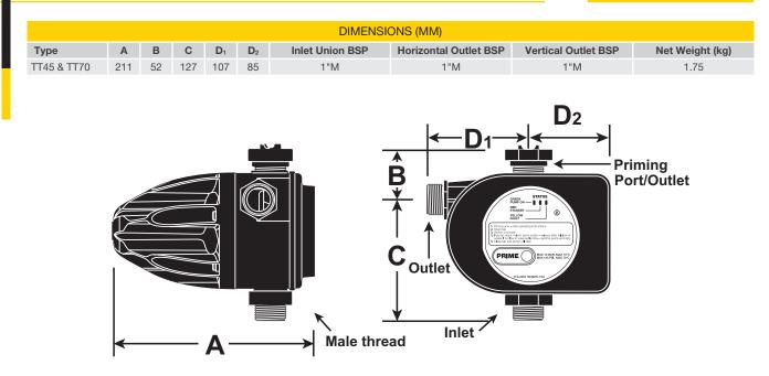
$^{\ast}$  Suction & delivery accept  $1^{1}\!/_{2}"$  PVC pipe on the I.D. and 2" fitting on the O.D.
