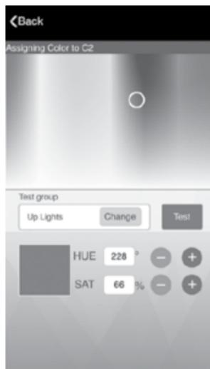
4. Select/confirm a color by dragging the circle selector to the desired color. Make changes in smaller increments by using the “+” and “-” buttons next to hue (horizontal) and saturation (vertical). The color is confirmed by the large color swatch.
